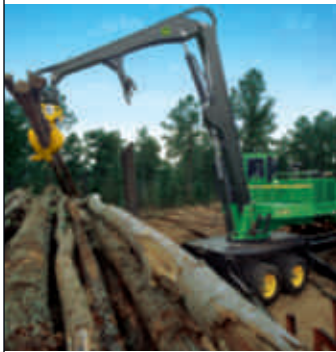
The 437C load-sense system features two-pump variable displacement with dedicated swing pump for significant reduction in fuel consumption and noise levels.
